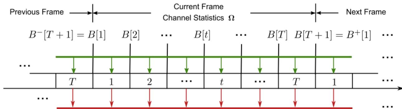
**Energy dynamics:**  $B[t+1] = \min(B[t] + G[t] - (E[t] - \tau P_r)^+, B_{\max})$ ;
