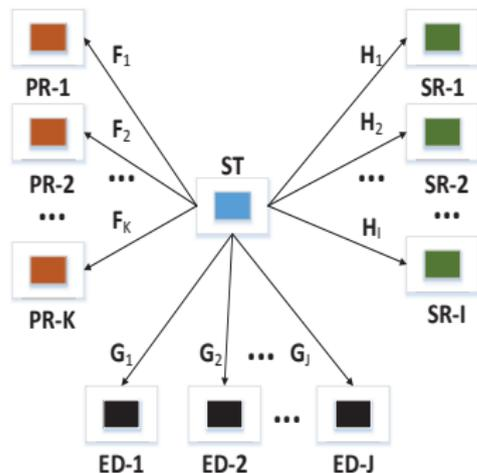
ST – secondary transmitter to design precoder  $\mathbf{P}$ ;
