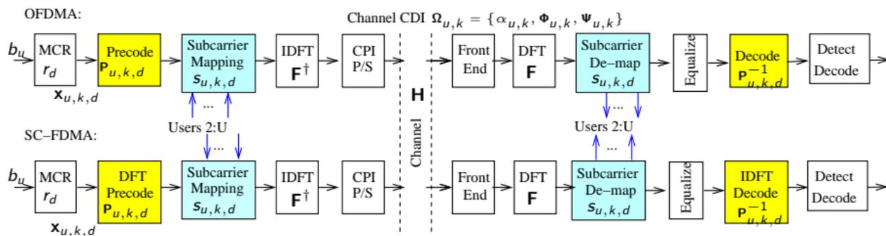
**Spectral efficiency**  $r_d = c_d \cdot N_t \cdot \log_2 M_d$ .
