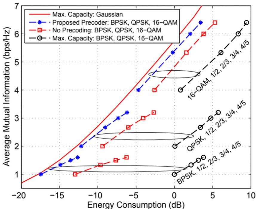
Energy consumption vs. AMI for  $2 \times 2$  correlated MIMO channels.
