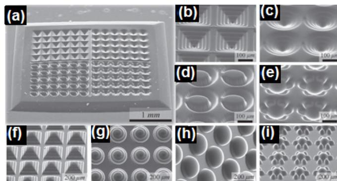
**Figure 3.** (a-i) SEM Images of the Fabricated 100%-PEGDA Microwells and Microarchitectures. Reprinted with permission from ref (24). Copyright 2012 John Wiley and Sons.
