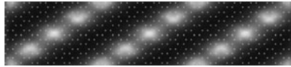
Fig. 1. Charge density induced on the surface of the [7, 0] zigzag nanotube in response to the potential of the phosphate groups of the DNA wrapped around the nanotube (gradient from gray to white/black corresponds to increasing positive/negative charge). Three unit cells are shown unfolded onto a plane.
