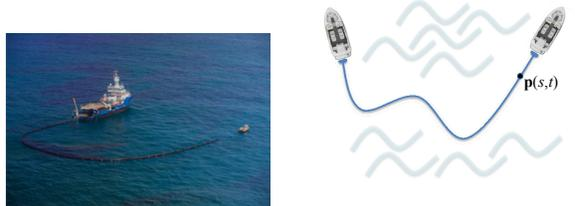
(a) A skimming operation with two vessels in the gulf of Mexico. (b) Two boats towing a rope.
