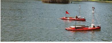
Fig. 5. A snapshot of one of the data-gathering trials. The two ASVs and the rope are visible. The markers had not been placed on the rope in this trial.
