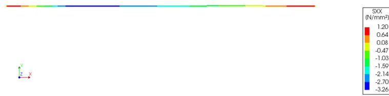
a) 1D: Beam elements
