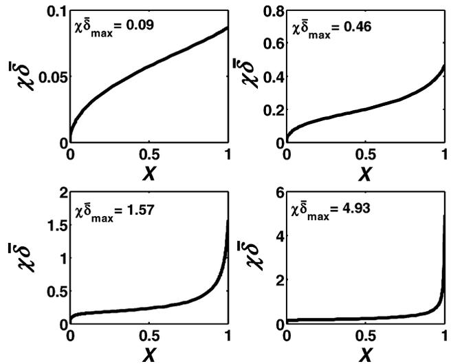
**Figure 8.** Normalized crack opening profiles versus normalized distance behind crack tip for different  $\chi \bar{\delta}_{\max}$ .
