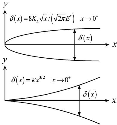
**Figure 3.** Two possible crack opening profiles. The top profile implies that there is energy flow to the crack tip, whereas there is no energy flow to the crack tip for the bottom profile.
