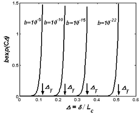
**Figure 4.** Dependence of rate of chain breakage on the stretch ratio for different  $b$  values.  $b^{-1} = 4\Sigma_0 k_s \tau_- V/n\pi E^*$  is the normalized velocity of crack propagation.  $C = k_s \lambda L_c/kT$ ,  $\Delta = \delta/L_c$  is the normalized crack opening displacement.  $\Delta_T$  (see (47)) corresponding to different  $b$  values is indicated.
