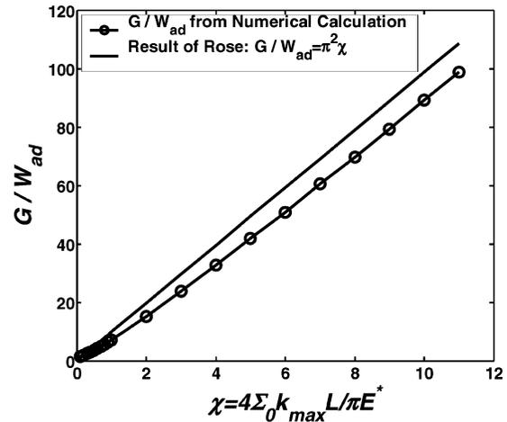
**Figure 7.** Relation between  $G/W_{ad}$  and the normalized cohesive zone length  $\chi$ . Circles (lower curve) represent numerical solutions. The upper curve is the approximate solution given by (A14).
