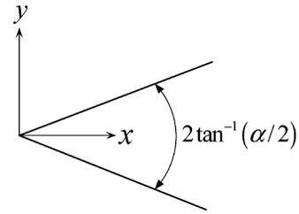
**Figure 2.** The crack opens up to a wedge with an internal angle  $2 \tan^{-1}(\alpha/2)$ .
