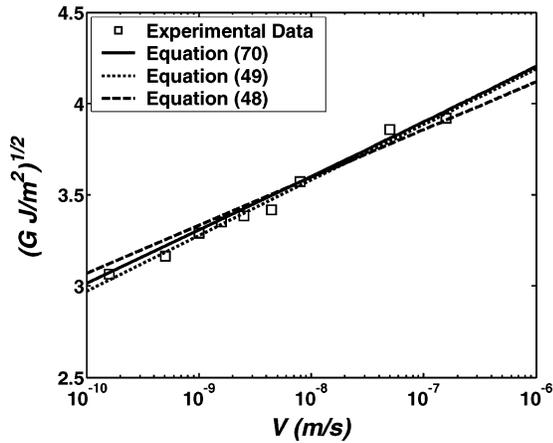
**Figure 6.** Comparison of three predictions of the energy release rate with experimental data.
