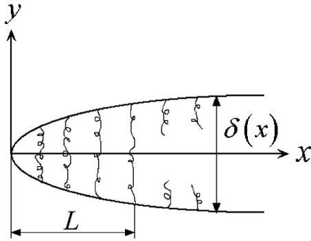
**Figure 1.** Crack with cohesive zone. The springs bridging the crack faces have a constant stiffness  $k_s$ . The stretch of the springs is denoted by  $\delta(x)$ , where  $x$  is the distance from the crack tip.  $L$  is the cohesive zone length.
