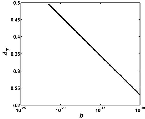
**Figure 5.** Normalized critical opening displacement  $\Delta_T$  vs normalized velocity  $b$ . Even for the smallest  $b = 10^{-22}$ , all the chains would have been broken when  $\Delta = \delta/L_c \approx 0.5$ .
