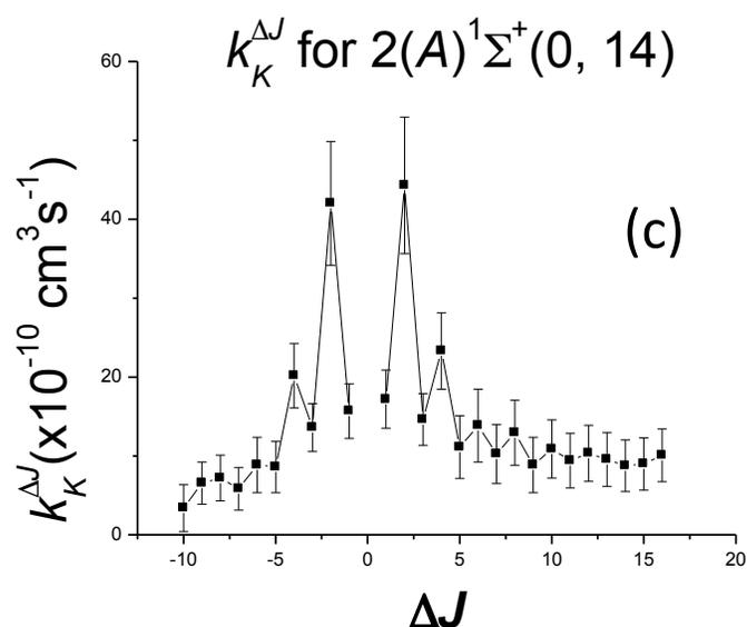
Supplementary Material Fig. 27: Rate coefficients for rotationally inelastic collisions of NaK  $2(A)^1\Sigma^+(v=0, J=14)$  molecules with (a) argon, (b) helium, and (c) potassium atoms as functions of  $\Delta J$ .
