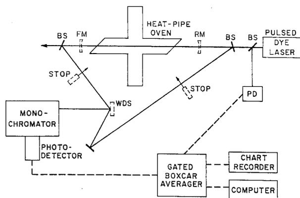
**Fig. 2.** Experimental set-up. Here PD, BS, RM, FM, and WDS represent photodiode, beam splitter, rear cavity mirror, forward cavity mirror, and white diffusing surface, respectively
