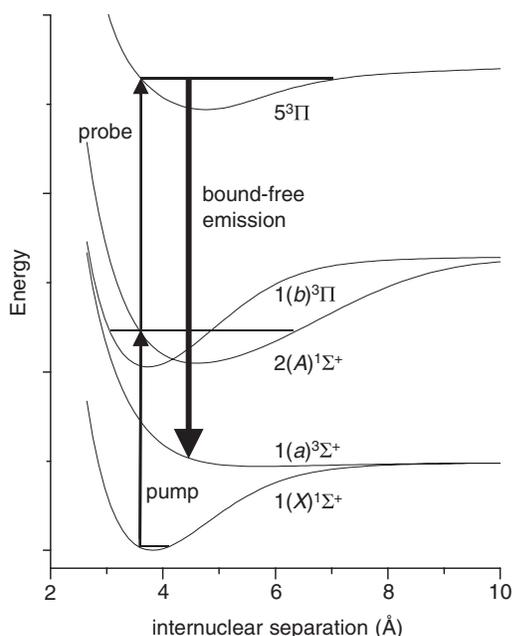
FIG. 2. PFOODR pump and probe scheme used to study the NaCs  $5^3\Pi_0$  and  $1(a)^3\Sigma^+$  states. The thick downward arrow indicates the  $5^3\Pi_0 \rightarrow 1(a)^3\Sigma^+$  bound-free emission.
