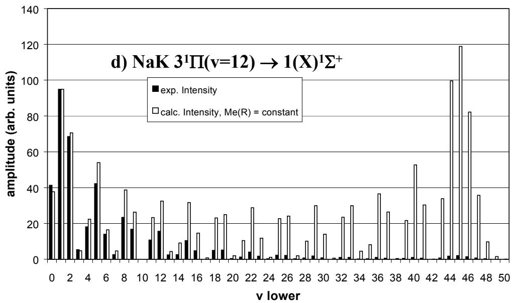
**Fig. 4 Revised.** Experimental and calculated relative intensities for transitions from  $3^1\Pi(v, J=30, f)$  to different  $1(X)^1\Sigma^+(v'', J=30, e)$  levels. (a)  $v = 6$ , (b)  $v = 8$ , (c)  $v = 10$ , (d)  $v = 12$ . In these calculations, the transition dipole moment was taken to be constant with internuclear separation. Experimental and calculated values are normalized to each other at the highest intensity experimental peak.
