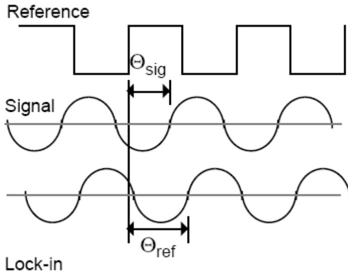
The signal is  $V_{sig}\sin(\omega_r t + \theta_{sig})$  where  $V_{sig}$  is the signal amplitude,  $\omega_r$  is the signal frequency, and  $\theta_{sig}$  is the signal's phase. Lock-in amplifiers generate their own internal reference signal usually by a phase-locked-loop locked to the external reference. In the diagram below the external reference, the lock-in's reference and the signal are all shown. The internal reference is  $V_L\sin(\omega_L t + \theta_{ref})$ .
