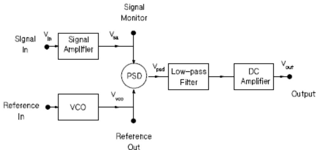
The signal to be measured is fed into the input of the AC Amplifier. The output of the DC amplifier is a DC voltage proportional to  $V_0$ . This voltage is displayed on the lock-in's own meter, and is also available at the output connector. I now elaborate on the functions of the five stages.
