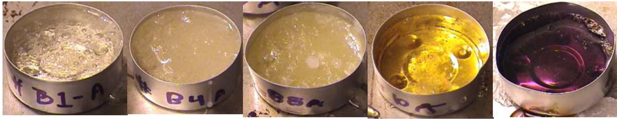
Fig. 6. Demonstration of increasing glass-forming ability with decreasing modifier content from left to right. Unstirred sugar+H<sub>2</sub>O samples from Experiment B(a). Sample #B1(a) is mostly liquid with a few crystals floating. The fraction of crystals increases in #B4(a) and #B8(a), the latter being mostly solid. #10(a) is mostly solid glass with a few crystalline regions. Finally, the last sample (#B12(a)) is just solid glass.
