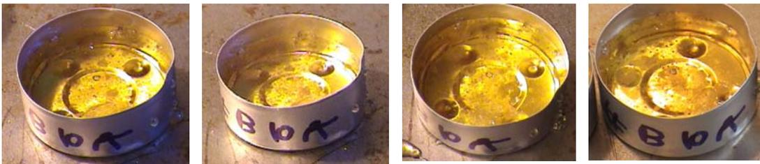
Fig. 5. Growth of sugar crystals in low modifier content mixture. The figure shows B10(a) sample with increasing time from left to right.
