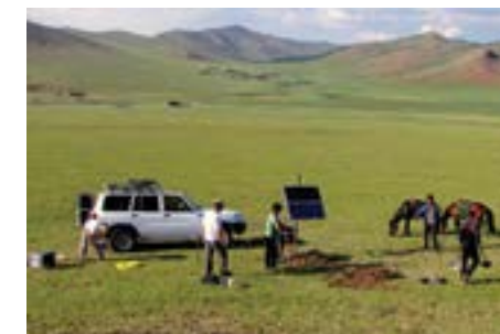
Researchers install a broadband seismic station at the Hangay Dome in central Mongolia. A family of "station keepers" watches over the security of the seismic station during the two-year recording period.
