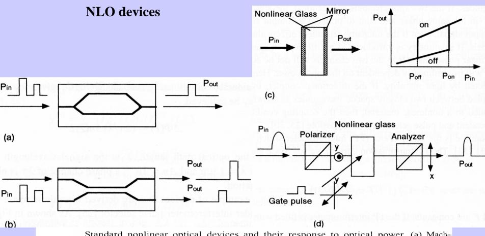
Standard nonlinear optical devices and their response to optical power, (a) Mach-Zehnder interferometer – pulse selector. (b) Nonlinear directional coupler. (c) Fabry-Pérot interferometer – bistable switching and (d) Optical Kerr shutter.
