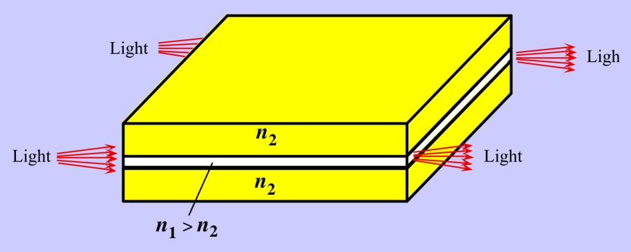
A planar dielectric waveguide has a central rectangular region of higher refractive index  $n_1$  than the surrounding region which has a refractive index  $n_2$ . It is assumed that the waveguide is infinitely wide and the central region is of thickness 2a. It is illuminated at one end by a monochromatic light source.
