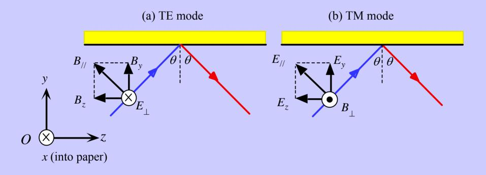
Possible modes can be classified in terms of (a) transelectric field (TE) and (b) transmagnetic field (TM). Plane of incidence is the paper.
