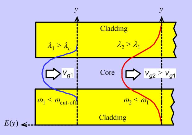
The electric field of  $TE_0$  mode extends more into the cladding as the wavelength increases. As more of the field is carried by the cladding, the group velocity increases.
