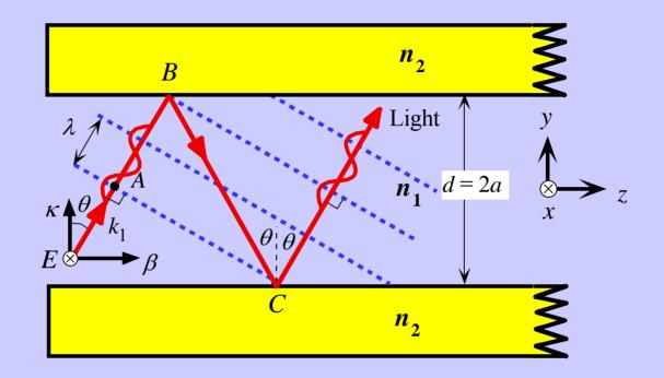
A light ray travelling in the guide must interfere constructively with itself to propagate successfully. Otherwise destructive interference will destroy the wave.
