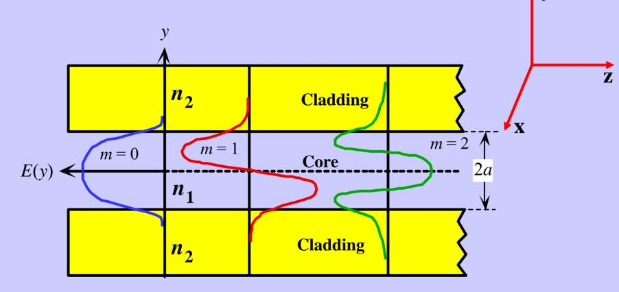
The electric field patterns of the first three modes (m = 0, 1, 2) traveling wave along the guide. Notice different extents of field penetration into the cladding. (Evanescent field increases with mode order and  $\lambda$ ). © 1999 S.O. Kasap, *Optoelectronics* (Prentice Hall)
