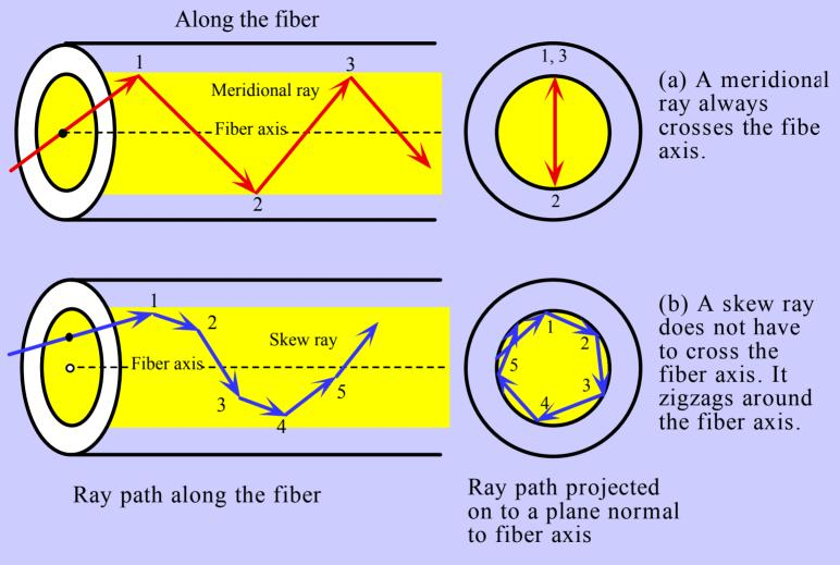
Illustration of the difference between a meridional ray and a <u>skew</u> ray. (Helical ray). Numbers represent reflections of the ray.
