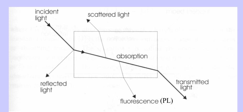
The interaction of light with a transparent material. The "bending" of the light ray on entering and leaving the material is called refraction and is discussed in Chapter 2. All of the processes labelled (reflection, absorption, scattering and fluorescence), can lead to colour production
