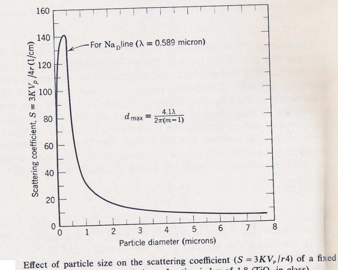
Effect of particle size on the scattering coefficient  $(3 - 3Kv_p/14)$  of a fixed volume of particles (1.0 vol%) for a relative refractive index of 1.8 (TiO<sub>2</sub> in glass).
