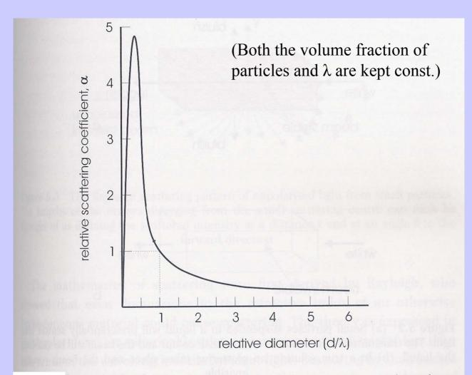
Schematic illustration of the effect of particle size, expressed as relative diameter (particle diameter, d / wavelength of light,  $\lambda$ ) on the relative scattering coefficient,  $\alpha$ , expressed as the ratio of the scattering coefficient  $\alpha_s$  at the relative diameter of 1.0 to that at other relative diameters. The maximum scattering occurs when the particle diameter is about half the wavelength of the light
