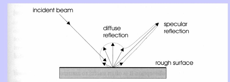
Reflection of light from a rough surface consists of two components, diffuse reflection and specular reflection. As the surface roughness increases the amount of diffuse reflection relative to the specular reflection increases. The ratio is an indication of surface gloss
