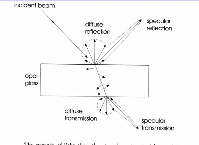
The passage of light through a translucent material containing many scattering centres, such as opal glass. Both the surface reflection and the transmitted light have diffuse and specular components
