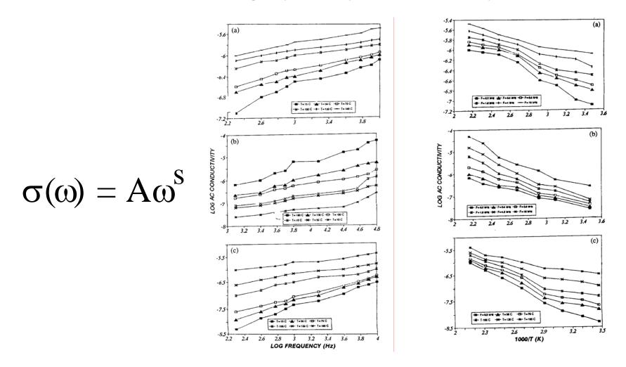
A.C .Electrical Conductivity Data of Tellurite Glasses containing MoO3 by ElKholy and ElMallawany (1995)
