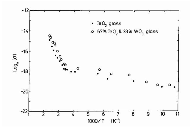
The D.C. electrical conductivity for the glassy systems in different temperature ranges and modifiers, by El-Mallawany at al, (1995)
