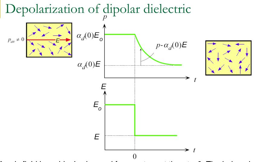
The dc field is suddenly changed from  $\mathcal{E}_o$  to  $\mathcal{E}$  at time t = 0. The induced dipole moment p has to decrease from  $\alpha_d(0)\mathcal{E}_o$  to a final value of  $\alpha_d(0)\mathcal{E}$ . The decrease is achieved by random collisions of molecules in the gas.
