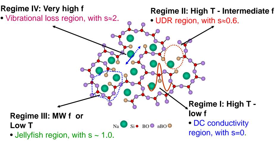
Random network structure of a sodium silicate glass in two-dimension (after Warren and Biscoe)
