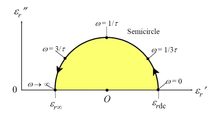
*Cole-Cole* plot is a plot of  $\varepsilon'_r$  vs.  $\varepsilon'_r$  as a function of frequency,  $\omega$ . As the frequency is changed from low to high frequencies, the plot traces out a circle if Debye equations are obeyed.
