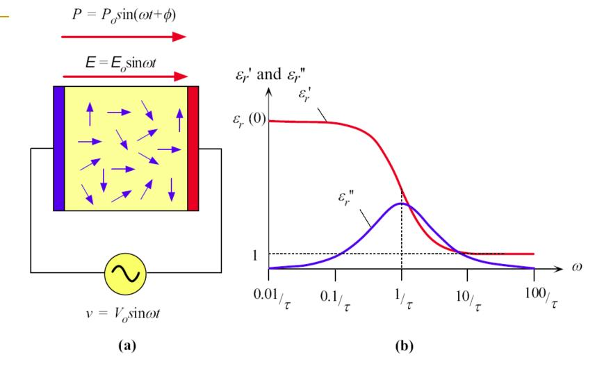
(a) An ac field is applied to a dipolar medium. The polarization P(P = Np) is out of phase with the ac field.
