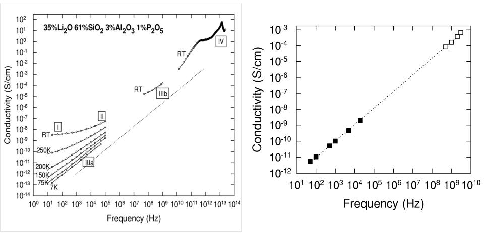
The source of dielectric loss (ac conductivity) at low T – low  $\omega$  and high T – MW  $\omega$  has a common underlying origin.
