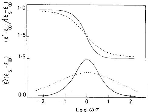
$\tau = \tau_0 \exp (Q/RT)$ where Q is activation energy for the reorientation of a dipole.
