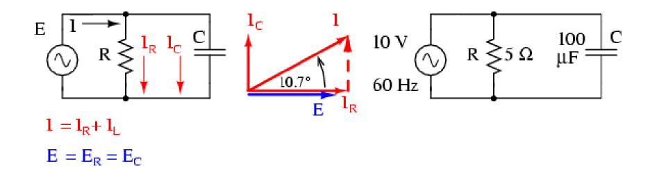
The total current can be considered as made of a lossy resistive component,  $I_L$  (or  $I_R$ ) that is in-phase with voltage, and a capacitive current,  $I_C$ , that is 90° out-of-phase.
