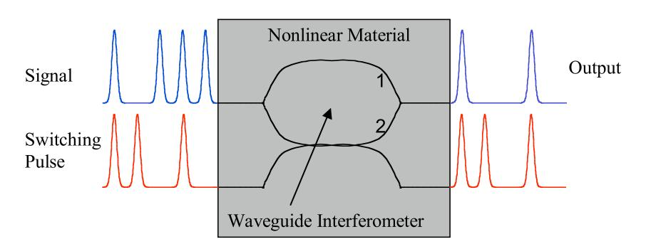
Without switching pulse: waves in leg 1 and 2 interfere destructively, no output
