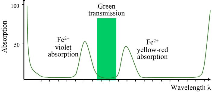
Because of electronic transitions involving the d orbitals, transition metals absorb visible light within the transparency window and produce colors. They are used as colorant in glasses. Crystal Field Theory: colors in glass and gems
