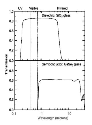
In a pure glass, the optical window is controlled by intrinsic limitations of the material : the electronic and vibrational transitions of the glass.
