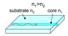
• Planar optical circuits permit to design compact devices for telecom network routing, optical sensing etc.. combining many optical components:
