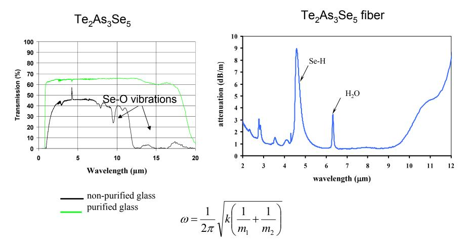
• Low mass impurities such as O or H generate phonon absorption peaks at lower wavelength within the transmission window of chalcogenide glasses.
