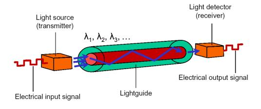
The current limitation to transmission rate is due to electronic signal routing which is slower than optical. All optical systems are therefore being developped.
