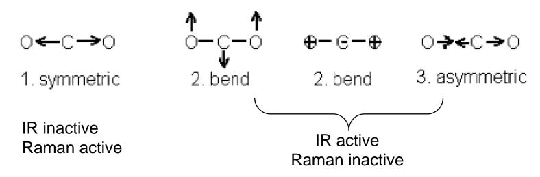
The CO<sub>2</sub> molecule has a center of symmetry located at the carbon atom and so obeys the exclusion rule, "In a centrosymmetric molecule no Raman-active molecule is also infrared-active and no infrared-active vibration is also Raman active."
