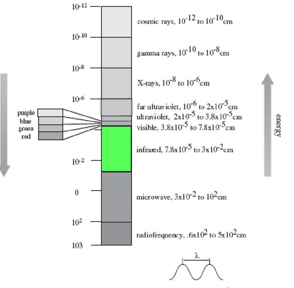
Infrared refers to that part of the electromagnetic spectrum between the visible and microwave regions.
