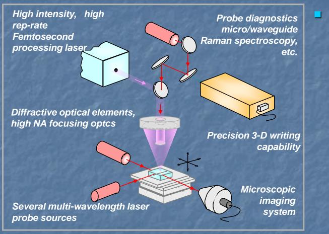
Goal: probe dynamic material response during laser writing to ascertain detailed knowledge of material modification mechanisms and kinetics
