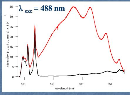
Fluorescence spectra (left) for modified (red) and unmodified (black) IOG-1 phosphate glass.  $\lambda_{exc}$  = 488 nm. Increase emission is attributable to formation of POHC defect upon illumination via proposed mechanism below.
