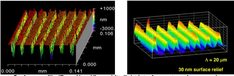
•Surface profile (Zygo New View white light interferometer microscope)
