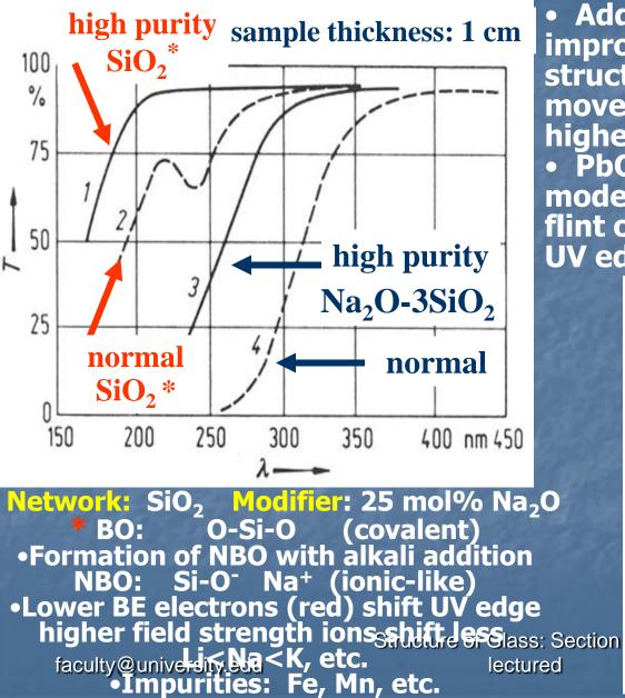
Additions of Al<sub>2</sub>O3 and B<sub>2</sub>O<sub>3</sub> improve the tetrahedral network structure, consuming NBO's and move the UV edge back up to higher frequencies.
