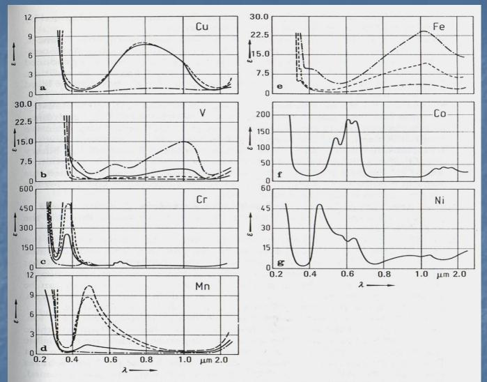
FIGURE 109a-g. Spectra of some transition elements in sodium silicate glasses, from Bamford [41, 42] ( $\varepsilon$  = molar normal extinction coefficient in 1/[mole cm]).
