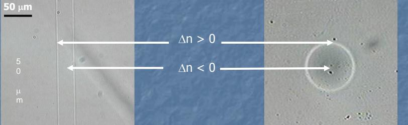
Annular refractive index distribution caused by thermal expansion in the focus - resolved by a DIC microscope
