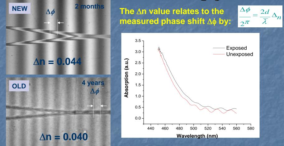
Aging to remove deposition-induced stress to yield stable, relaxed network structure <u>does not adversely affect resulting film photosensitivity</u>.
