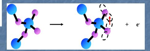
Proposed mechanism for the production of phosphorus-oxygen hole center (POHC) defects. The precursor consists of two nonbridging oxygen (NBO) atoms (pink) connected to a phosphorus (blue) atom, a defect that is common in phosphate glasses. A hole gets trapped on two orbitals of the two oxygen atoms to form the fac POHC. Resulting index change in exposed region of the glass is (-). 46
