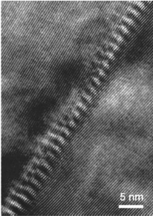
Figure 1. HRTEM of grain boundary in 1.0 mol % Y<sub>2</sub>O<sub>3</sub>-doped CeO<sub>2</sub>. The moiré rings are also visible.
