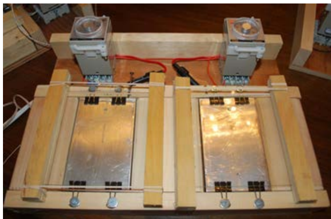
Figure 1. Dual temperature controlled sample “hot plate oven” made from 75 W strip heater ($30, McMaster-Carr) bolted to a ¼”x3”x5” aluminum plate and controlled with the Autonics TOS Analog controller. Samples are covered with a glass plate enclosure above the sample to simulate an oven (plate IS shown here).
