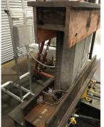
One project being carried out by the TES team is for a sensible heat TES concept that utilizes cementitious materials with enhanced thermomechanical properties for this type of application. Prof. Clay Naito says, "Dissimilar thermal expansion between thermosiphons, which charge the media, and concrete can result in the formation of high tensile
