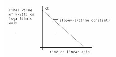
If the upper left part of your plot tails away from a straight line it is likely that your plant is better represented by a second-order transfer function. In MEM1 this should not happen, or at least it should not be significant. Simple as it is, this is a typical identification problem with the plant transfer function assumed *a priori*.
