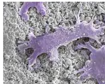
A scanning electron micrograph of a bone cell (pseudocolored in purple) attached to the surface of a TAMP scaffold that is useful for regenerating new tissue.
