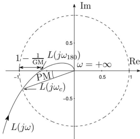
**Figure 6:** Typical Nyquist plot of  $L(j\omega)$  for stable plant with PM and GM indicated. Closed-loop instability occurs if  $L(j\omega)$  encircles the critical point  $-1$ .
