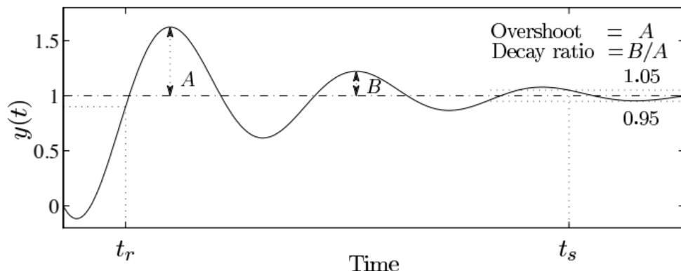
**Figure 5:** Step response analysis: Rise time ( $t_r$ ), Settling time ( $t_s$ ), Overshoot ( $A$ ), Peak time ( $t_p$ ), Decay Ratio ( $B$ ), Steady-state Offset, Total Variation.
