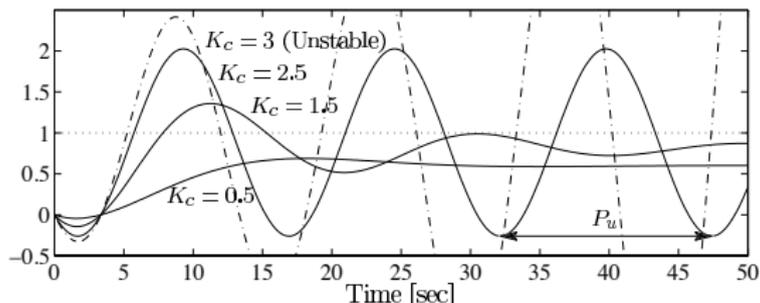
Figure 2: Effect of proportional gain  $K_c$  on closed-loop response  $y(t)$ .
