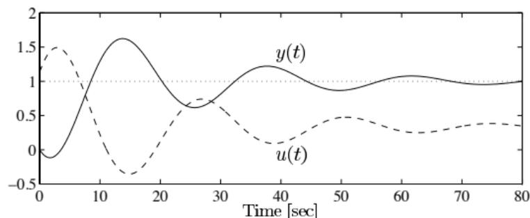
Figure 3: Closed-loop step response  $y(t)$  with PI control.
