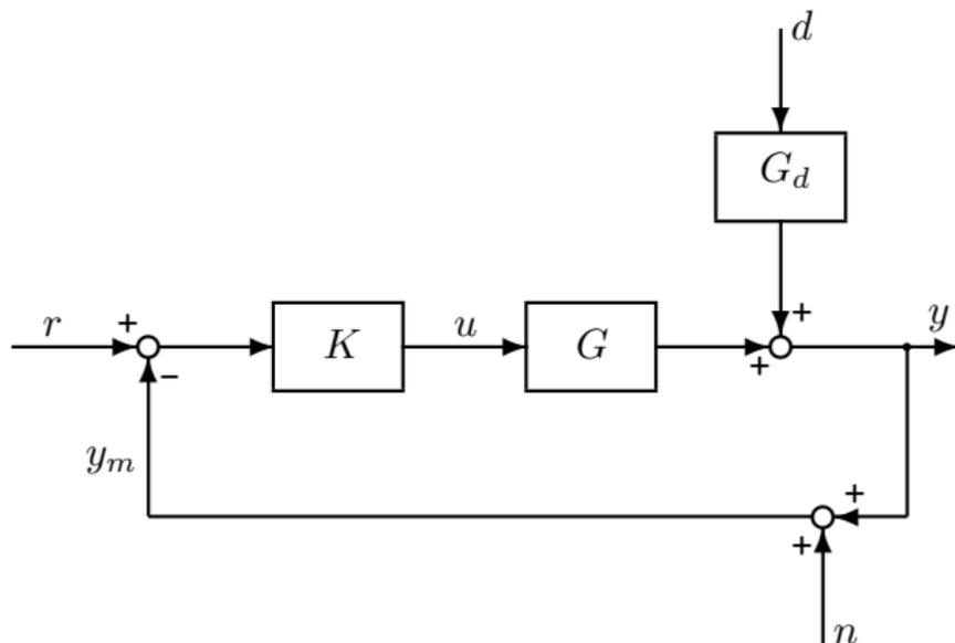
Figure 1: Block diagram of one degree-of-freedom feedback control system
