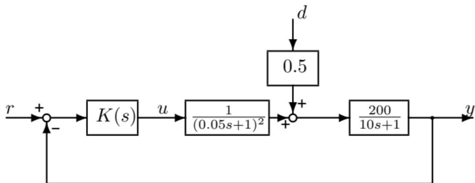
**Figure 8:** Block diagram representation of the disturbance process in (2.25)
