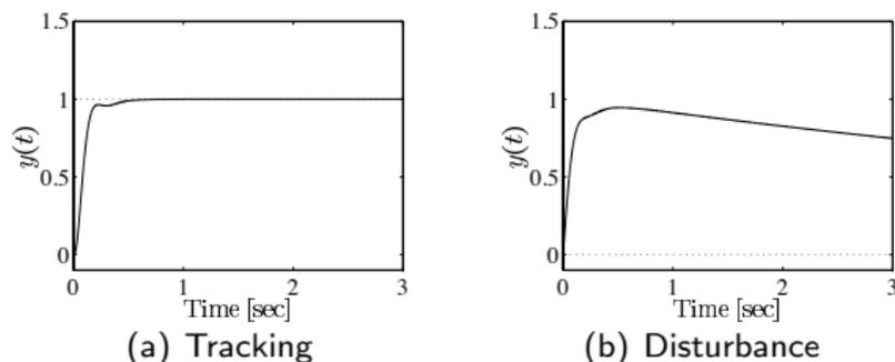
**Figure 7:** Responses with “inverse-based” controller  $K_0(s)$  for the disturbance process. Note excellent tracking response but poor disturbance-rejection response.
