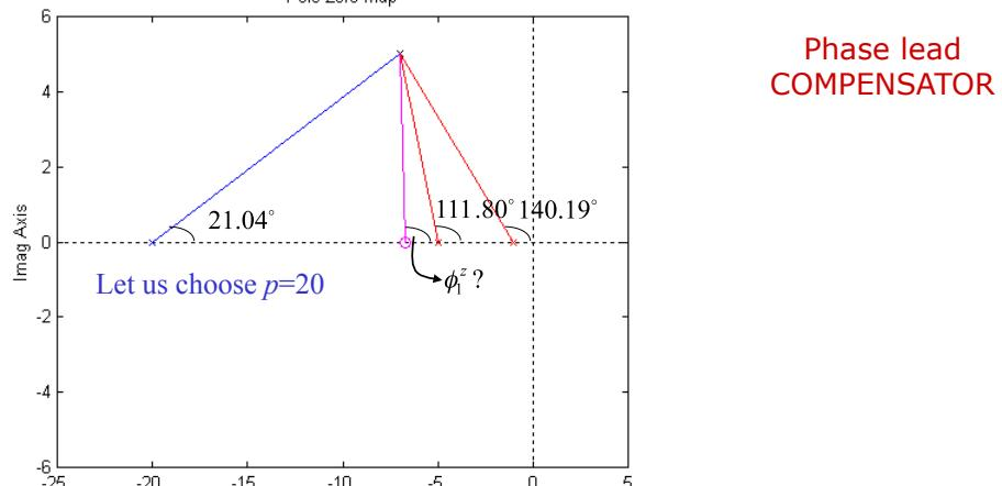
$$\angle L(s) = \phi^{K_p} + (\phi_1^z + \phi_2^z + \dots + \phi_m^z) - (\phi_1^p + \phi_2^p + \dots + \phi_n^p) = 180^\circ$$
