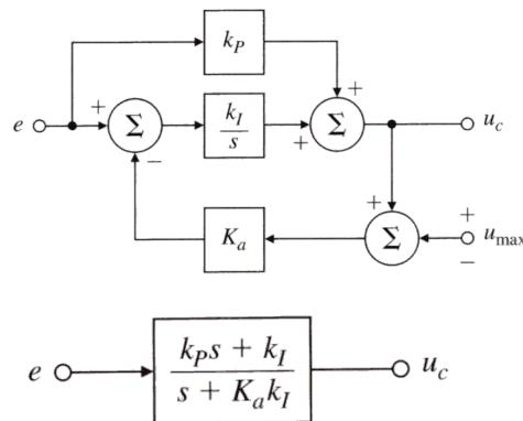
For large  $K_a$ , this is a system with very low gain and very fast decay rate, i.e., the integration is turned off.
