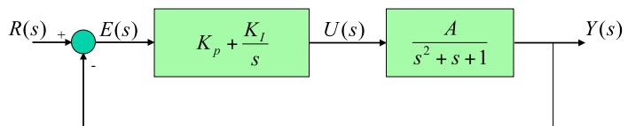
$$\frac{Y(s)}{R(s)} = \frac{\left( K_p + \frac{K_I}{s} \right) G(s)}{1 + \left( K_p + \frac{K_I}{s} \right) G(s)} = \frac{\left( K_p s + K_I \right) A}{s^3 + s^2 + (1 + K_p A)s + K_I A}$$
