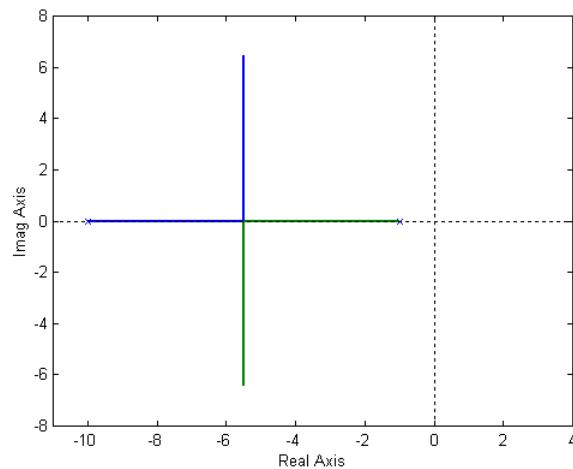
We need a systematic approach to plot the closed-loop poles as function of the gain  $K \rightarrow$  ROOT LOCUS
