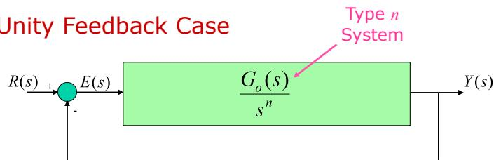
$$C(s)G(s) = \frac{G_o(s)}{s^n}, E(s) = \frac{1}{1 + \frac{G_o(s)}{s^n}} R(s), R(s) = \frac{1}{s^{k+1}}$$
