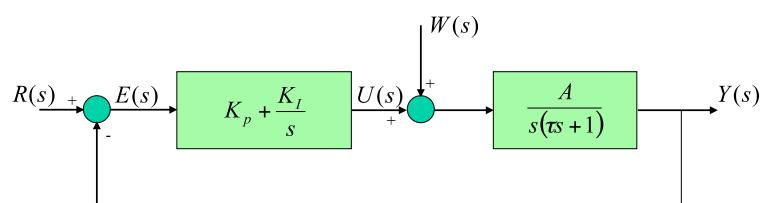
$$K_I \neq 0 \quad \Rightarrow \quad \text{type 1 to } w$$
