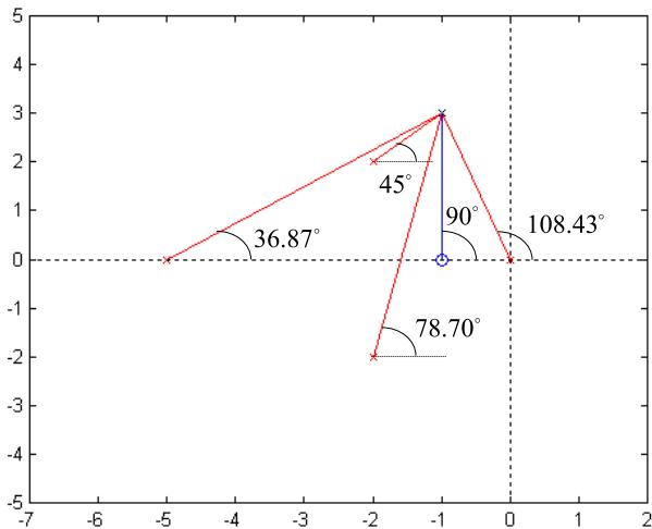
$$90^\circ - [108.43^\circ + 36.87^\circ + 45^\circ + 78.70^\circ] \approx -180^\circ \Rightarrow s_o = -1 + 3i \text{ belongs to the locus!}$$
