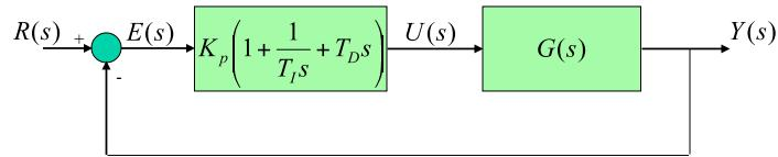
$$u(t) = K_p \left[ e(t) + \frac{1}{T_I} \int_0^t e(\tau) d\tau + T_D \frac{de(t)}{dt} \right] \quad K_I = \frac{K_p}{T_I}, \quad K_D = K_p T_D$$
