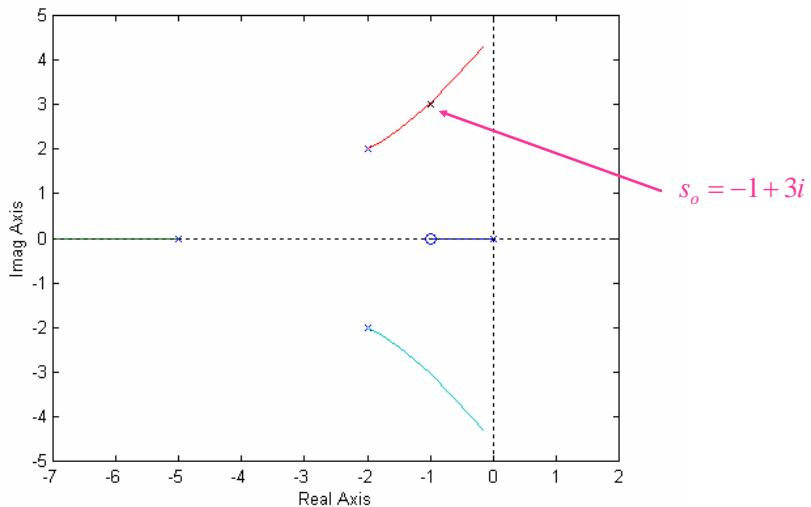
We need a systematic approach to plot the closed-loop poles as function of the gain  $K \rightarrow$  ROOT LOCUS
