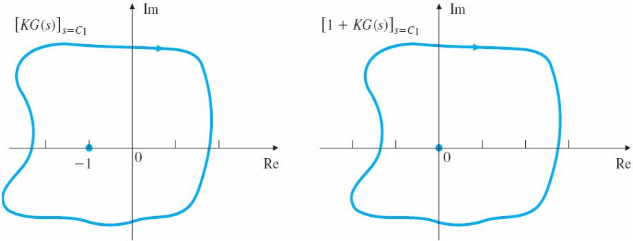
If the plot of  $1 + KG(s)$  encircles the origin, the plot of  $KG(s)$  encircles -1 on the real axis.
