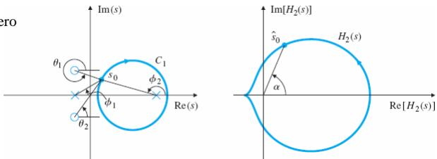
**Argument Principle:** A contour map of a complex function will encircle the origin  $Z$ - $P$  times, where  $Z$  is the number of zeros and  $P$  is the number of poles of the function inside the contour.
