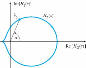
**Argument Principle:** A contour map of a complex function will encircle the origin  $Z$ - $P$  times, where  $Z$  is the number of zeros and  $P$  is the number of poles of the function inside the contour.
