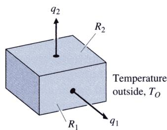
$$\dot{T}_I = \frac{1}{C_I} \left( \frac{1}{R_1} + \frac{1}{R_2} \right) (T_o - T_I)$$
