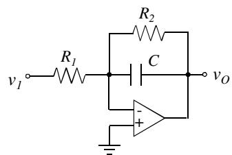
$$\frac{dv_O}{dt} = \frac{1}{R_2 C} v_O - \frac{1}{R_1 C} v_I$$
