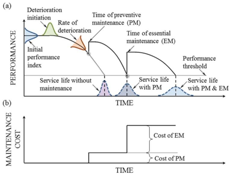
*Deterioration and maintenance effects on performance and cost*
