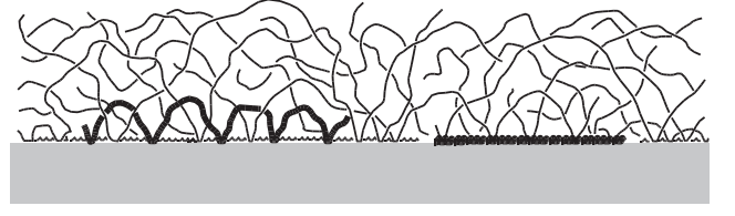
Fig. 10. Sketch of predicted final layer structure resulting from irreversible polymer adsorption. The layer consists of two parts (one chain from each part is highlighted): i) An inner region of flattened down chains making \omega N contacts per chain, where \omega is of order unity. ii) A diffuse outer layer build-up from chains each making fN \ll N contacts with the surface. The values of f follow a distribution P(f) \sim f^{-4/5} . Each f value corresponds to a characteristic loop size for a given chain, s \approx n_{\text{cont}}/f .
