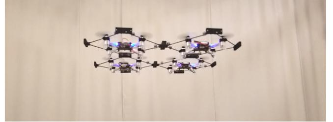
(a) Four docked modules in a  $2 \times 2$  configuration
