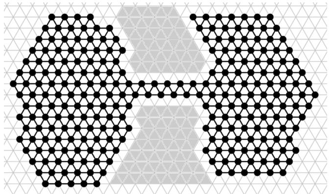
Fig. 9. A robot formation in a triangular lattice. This special configuration can take advantage of the boundary properties to reduce the required communication radii. The robustness of the formation shown can be guaranteed by using the appropriate communication range of: a connected formation, a triangular formation, or a heterogeneous communication radii. The lattice length is  $\ell = 1$ .
