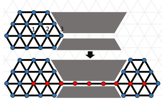
Fig. 6. Robots of different communication range can be used to deal with obstacles in the environment and optimize energy usage in the communications. The dots in red represent robots with a communication radius  $R_-(3)$ , while the ones in blue have  $R_Δ(3)$ . The formation is 3-robust.
