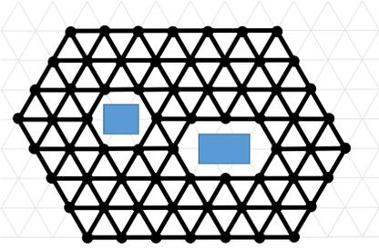
Fig. 4. Robots on a triangular lattice surrounding obstacles. The robots and the obstacles are depicted in black and blue respectively.
