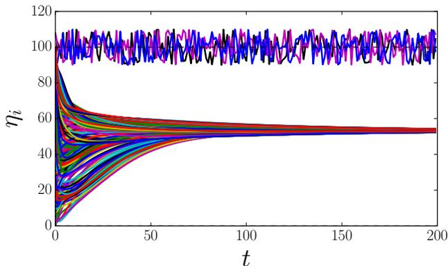
Fig. 11. Achieving consensus in a heterogeneous network of 398 robots and 4 malicious robots for the formation in Figure 9. The malicious robots share random values with mean 100, both inside and outside of the convex hull of the initial values.
