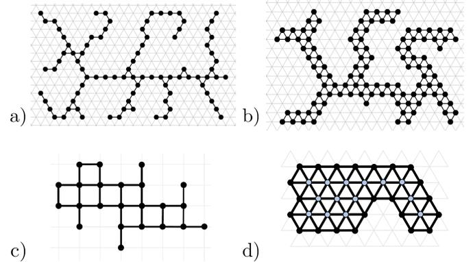
Fig. 1. Examples of robot formations: a) connected formation, b) triangular formation, c) square formation, d) formation with heterogeneous communication radii. The robots with large and small communication range are depicted in black and light blue, respectively.
