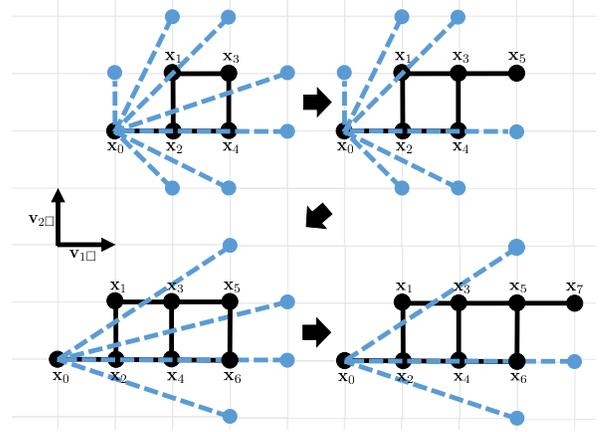
Fig. 3. Sequential addition of robots in a square lattice. Each subsequent robot in the formation is placed maximizing the distance from robot 0. The pattern repeats for all the successive robots.
