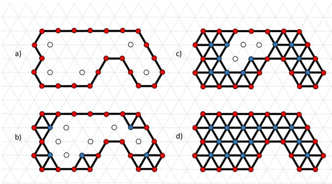
Fig. 7. A 3-robust formation of robots, depicted as black circles, surrounds an empty region on a triangular lattice. New robots can be added while preserving the robustness at the locations with blue circles. The sequence of images from a) to d) show how the region can be filled.
