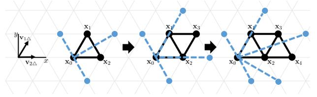
Fig. 2. The construction of a triangular formation that maximizes the distance from the first allocated robot. This shows how every subsequent robot in the formation is selected as to maximize the distance from robot 0 to the next robot. The blue lines denote the lattice locations where the next robot can be placed.
