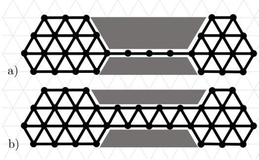
Fig. 5. Two sets of robots are connected through a narrow passage between obstacles. a) A connected formation with  $R = R_-(3F)$  is used. b) A locally triangular formation with  $R = R_Δ(3F + 1)$  is used, requiring more robots, but smaller communication range.
