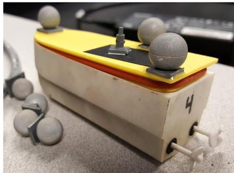
Fig. 4. A robotic boat driven by two propellers in the back. The reflective markers on the top are used for localization. A sealing system prevents water from entering the boat
