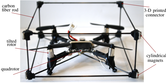
Fig. 2. A Flying Modular Robot. Equipped with cylindrical magnets located at the corner of the carbon fiber cages. This docking mechanism allows a one DOF connection between two modules.
