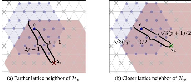
**Fig. 2** The farther and the closer neighbors of the centroid of  $\mathcal{H}_p$ . The blue disks represent the robots in  $\mathcal{H}_p$ . The x marks represent the lattice neighbors of  $\mathcal{H}_p$ . The red and blue X represent the farther and closer neighbors respectively. The red shadowed area represents the communication coverage of the neighbor for  $R = 2p - 1$ .
