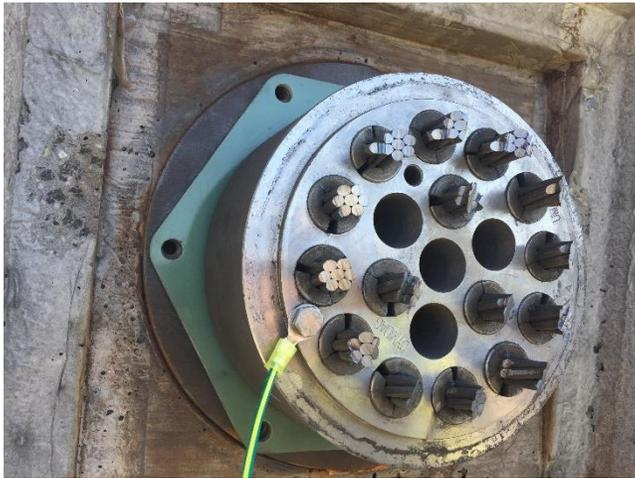
Measuring cable to wedge plate
