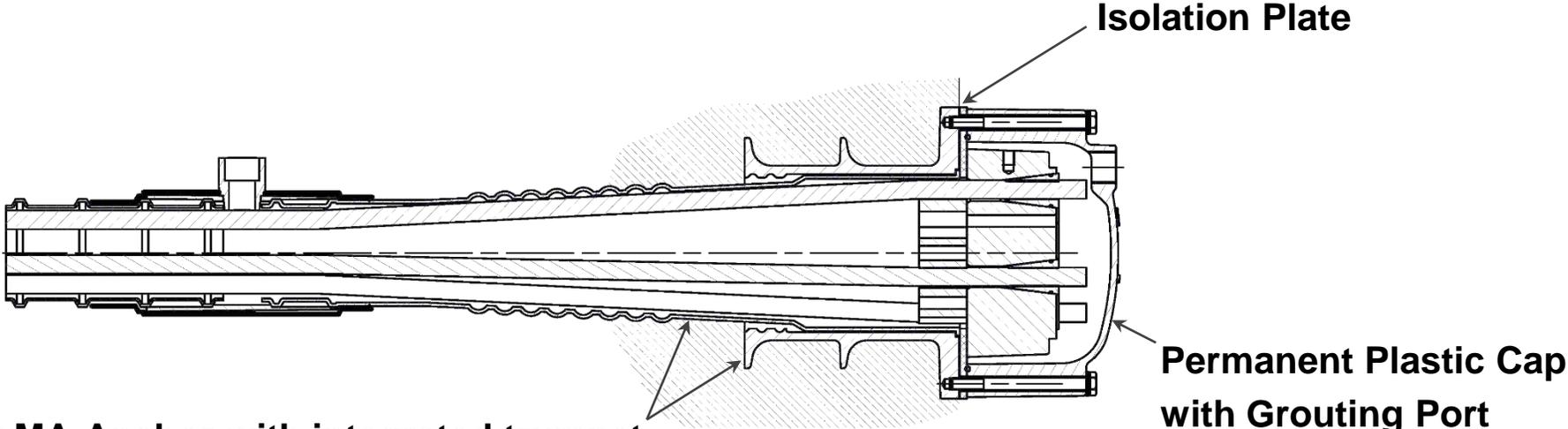
**New MA-Anchor with integrated trumpet**
