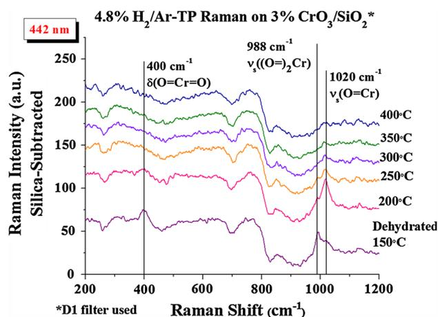
**Fig. 5** In situ TP-Raman spectroscopy of 3%  $CrO_3/SiO_2$  in 4.8%  $H_2/Ar$  after subtracting the silica support spectrum. The 3%  $CrO_3/SiO_2$  catalyst was heated to 500 °C at 10 °C/min in 10%  $O_2/Ar$ , held at 500 °C for 1 h, and cooled to 150 °C. It was then flushed for 30 min in  $Ar$ . Then the temperature was ramped to 500 °C in 4.8%  $H_2/Ar$ . Spectra were taken every 50 °C with the 442 nm laser and a D1 filter
