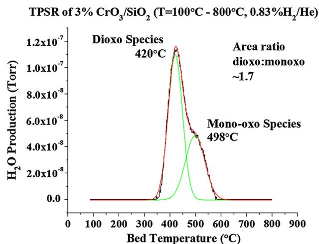
**Fig. 6** H<sub>2</sub>-TPSR of 3 wt% CrO<sub>3</sub>/SiO<sub>2</sub>. The 3 % CrO<sub>3</sub>/SiO<sub>2</sub> catalyst was heated to 500 °C at 10 °C/min in 10 % O<sub>2</sub>/Ar, held at 500 °C for 1 h, and cooled to 150 °C. It was then flushed with UHP He. Then the temperature was ramped to 800 °C in 0.83 % H<sub>2</sub>/He. H<sub>2</sub>O production was monitored
