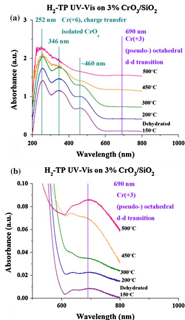
**Fig. 4** In situ  $H_2$  TP-UV-vis DRS of 3%  $CrO_3/SiO_2$  (a) full spectrum and (b) zoomed in to see the  $Cr^{+3}$  band. The 3%  $CrO_3/SiO_2$  catalyst was heated to 500 °C at 10 °C/min in 10%  $O_2/Ar$ , held at 500 °C for 1 h, and cooled to 150 °C. It was then flushed for 30 min in  $Ar$ . Then the temperature was ramped to 500 °C in 4.8%  $H_2$ . Spectra were taken every 50 °C
