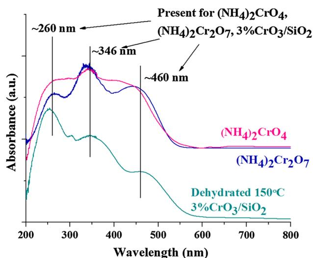
Fig. 2 UV-vis of reference compounds under ambient conditions
