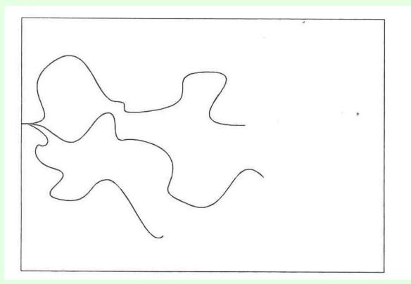
High Stress: Multiple crack surfaces were needed to absorb excessive energy.
