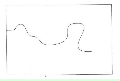
Low Stress: Single crack suggests a weaker glass edge. Less energy was needed to propagate the crack
