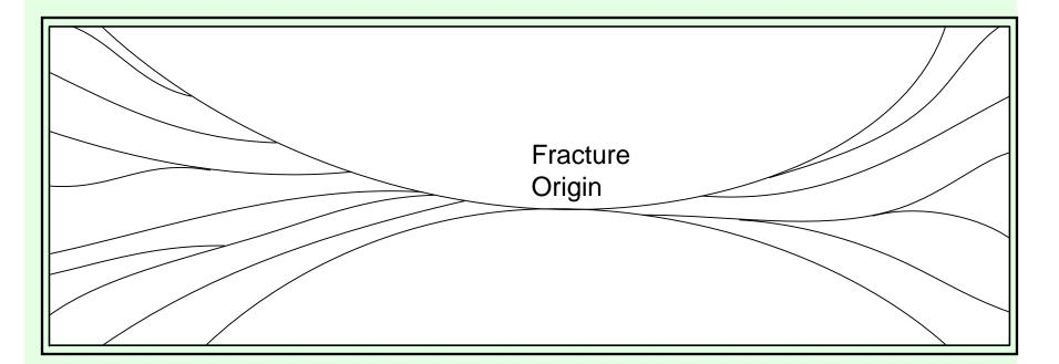
Properly glazed High Aspect Ratio Sealed Insulating Glass.
