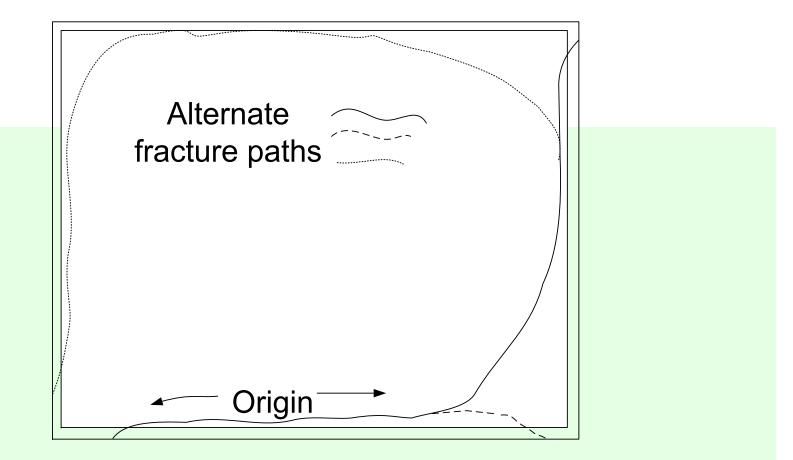
Incorrect 'Clamped Edges' create very high bending stresses at low temperatures in Insulating Glass. Fracture origin at a scratch.
