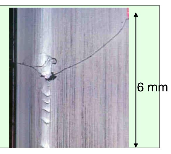
Fracture Origin at rub mark on IG cut edge. Thermal stress caused the small vent to run
