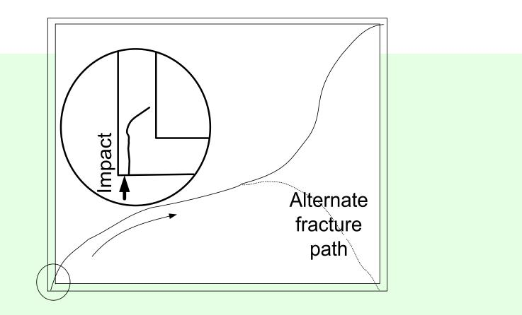
A corner impact easily creates a 10 or 20 mm long crack which waits for a high stress situation to make it run. Here low winter temperature contracts the sealed air space and creates a large bending stress.
