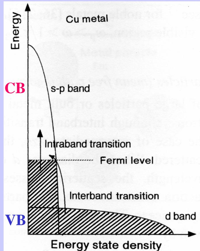
Schematic expression of electron state density and band structure of Cu metal.
