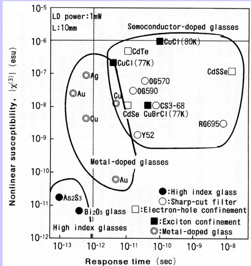
The nonlinear susceptibilities versus nonlinear response time. (Data from Table 4.4, 4.5, 4.6 and 4.7. The broken lines (response time:  $10^{-12}$  sec,  $|\chi^{(3)}|$ :  $10^{-6}$  esu) indicate the conditions required for obtaining  $2\pi$  phase shift when pulse selector is made using 1 mW-LD and 10 mm optical path [265].)
