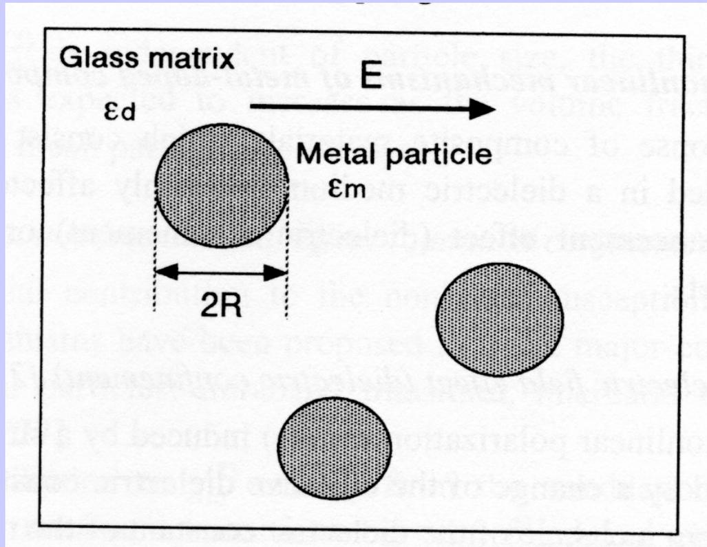
Schematic diagram of a composite material consisting of a metal particles of radius  $R$  with complex dielectric constant  $\epsilon_m$  embedded in a dielectric matrix with a real dielectric constant  $\epsilon_d$ .
