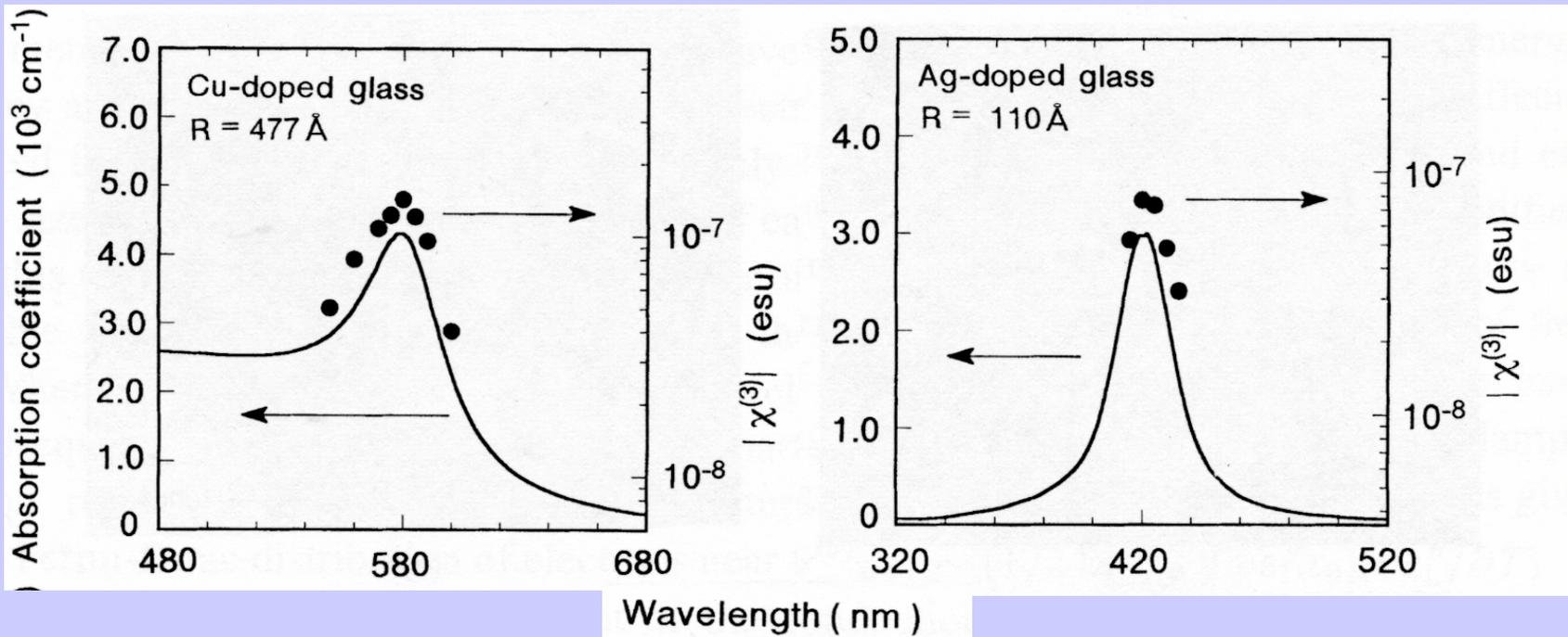
Absorption spectra and wavelength dependence of  $\chi^{(3)}$  for Cu- and Ag-doped glasses. [Reprinted from K. Uchida, S. Kaneko, S. Omi, C. Hata, H. Tanji, Y. Asahara, *et al. J. Opt. Soc. Am. B11* (1994) 1236, copyright (1994) with permission from the Optical Society of America.]
