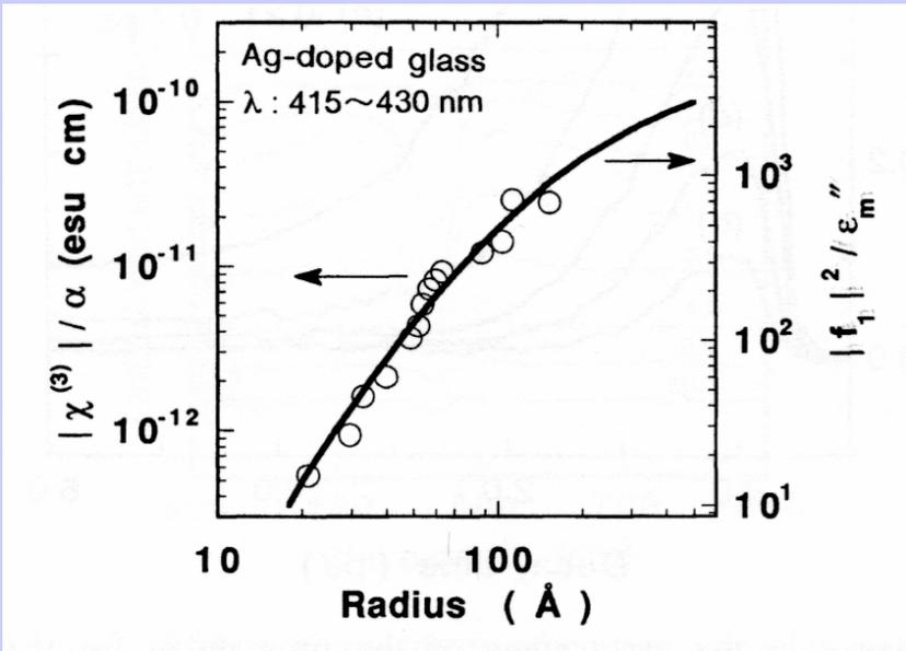
$\chi^{(3)}/\alpha$  and  $f_1^2/\epsilon_m''$  as a function of particle size. [Reprinted from K. Uchida, S. Kaneko, S. Omi, C. Hata, H. Tanji, Y. Asahara, *et al. J. Opt. Soc. Am.* **B11** (1994) 1236, copyright (1994) with permission from the Optical Society of America.]
