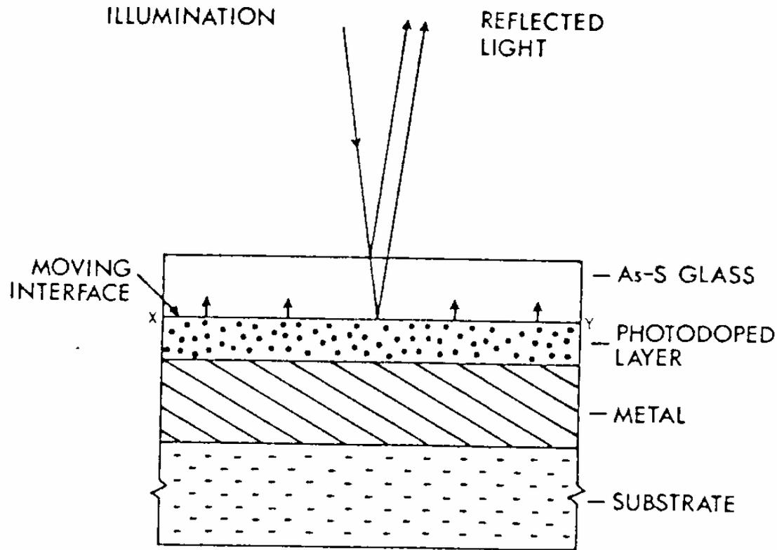
A schematic cross-section through a sample during the photodissolution process. Under illumination, metal ions dissolve into the As-S glass to form a new 'photodoped' material. The photodoped layer continues to grow as long as the sample is illuminated. The light stimulating the process is believed to be absorbed in the photodoped layer close to the interface X-Y.
