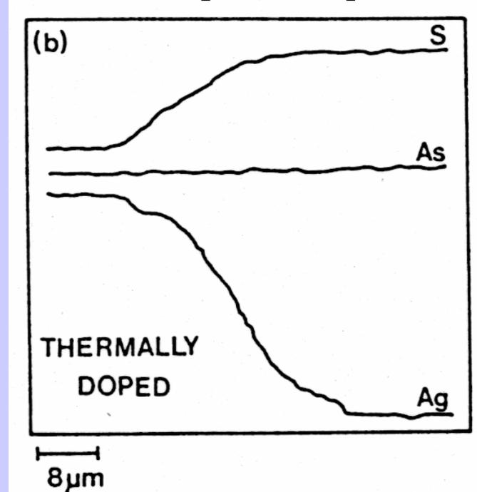
Ag and S concentration profiles (relative to As) in Ag-doped a-As<sub>2</sub>S<sub>3</sub> obtained by electron microprobe X-ray analysis (Matsuda and Kikuchi, 1973); (a) is for photodoped material and shows the 'step-like' Ag profile; (b) is for thermally doped material and shows a more gradual variation in Ag concentration in the interface region between the doped and undoped materials.
