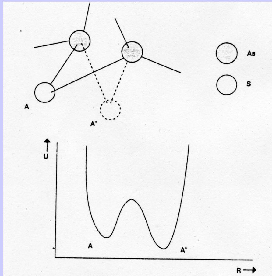
A schematic model of bistable bonding geometries in  $a\text{-As}_2\text{S}_3$  and the corresponding double-well potential. A and A' represent atomic configurations before and after illumination, R is some configurational coordinate and U the potential.
