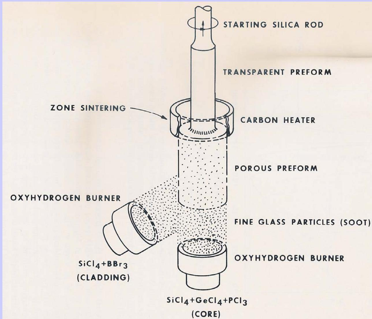
Illustration of vapor axial deposition process (VAD process). (Final drying step with  $\text{Cl}_2$ ).
