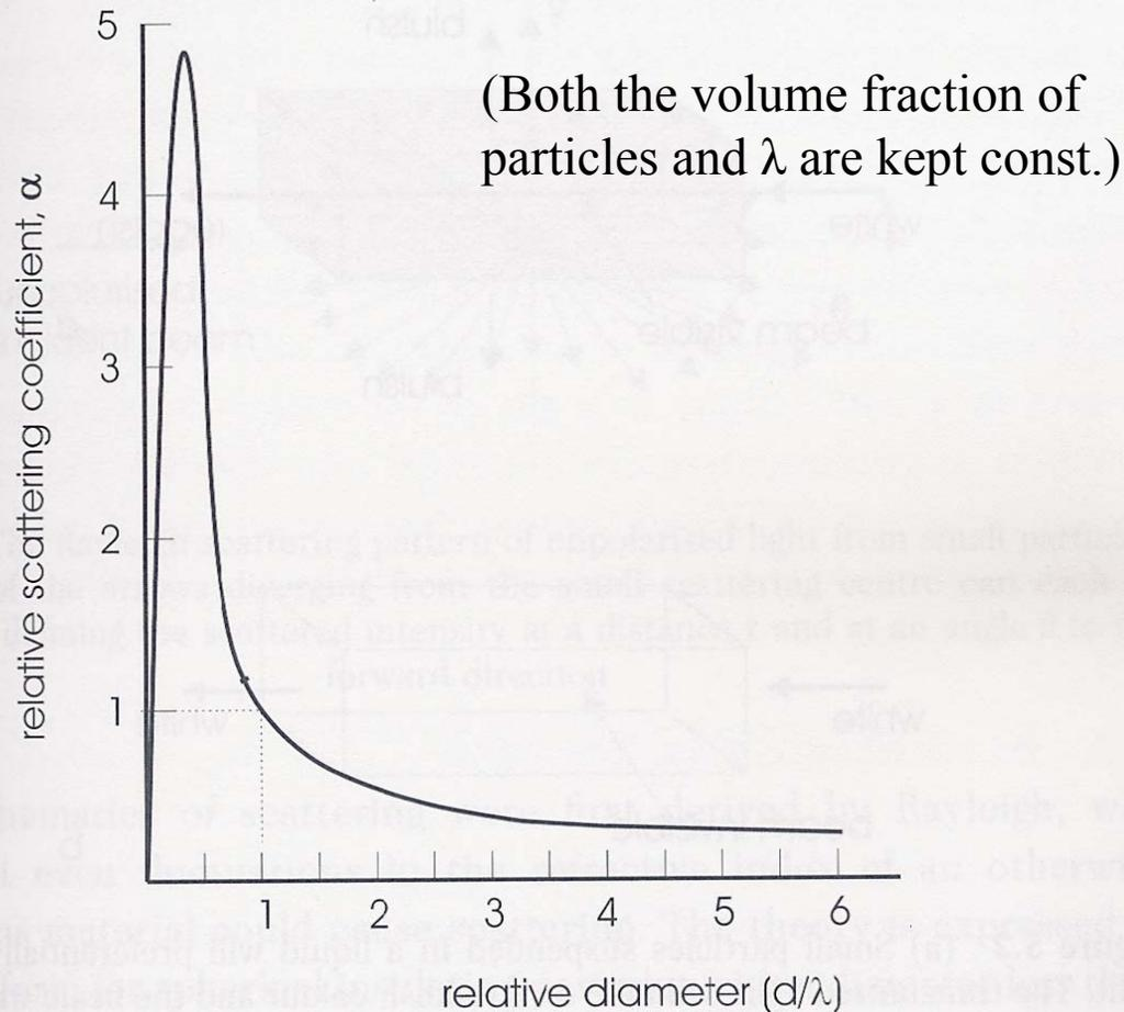
Schematic illustration of the effect of particle size, expressed as relative diameter (particle diameter,  $d$  / wavelength of light,  $\lambda$ ) on the relative scattering coefficient,  $\alpha$ , expressed as the ratio of the scattering coefficient  $\alpha_s$  at the relative diameter of 1.0 to that at other relative diameters. The maximum scattering occurs when the particle diameter is about half the wavelength of the light
