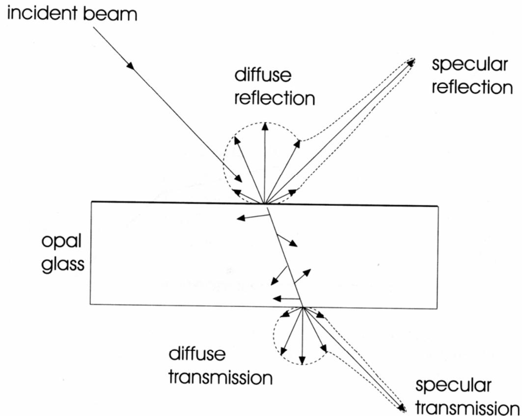
The passage of light through a translucent material containing many scattering centres, such as opal glass. Both the surface reflection and the transmitted light have diffuse and specular components
