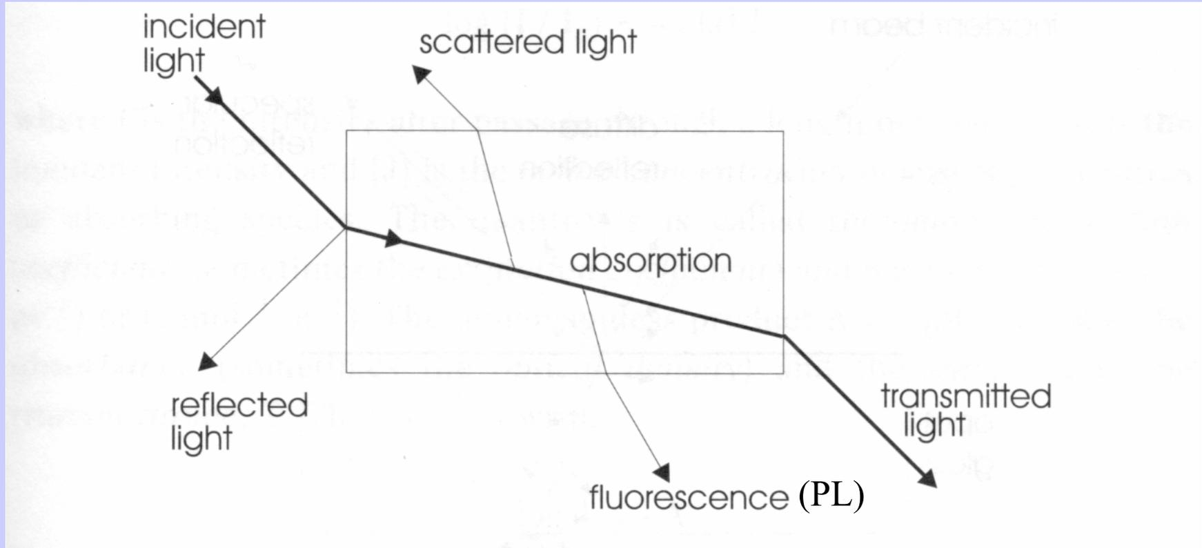
The interaction of light with a transparent material. The “bending” of the light ray on entering and leaving the material is called refraction and is discussed in Chapter 2. All of the processes labelled (reflection, absorption, scattering and fluorescence), can lead to colour production
