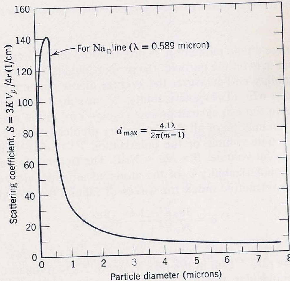
Effect of particle size on the scattering coefficient ( $S = 3KV_p / r4$ ) of a fixed volume of particles (1.0 vol%) for a relative refractive index of 1.8 (TiO<sub>2</sub> in glass).
