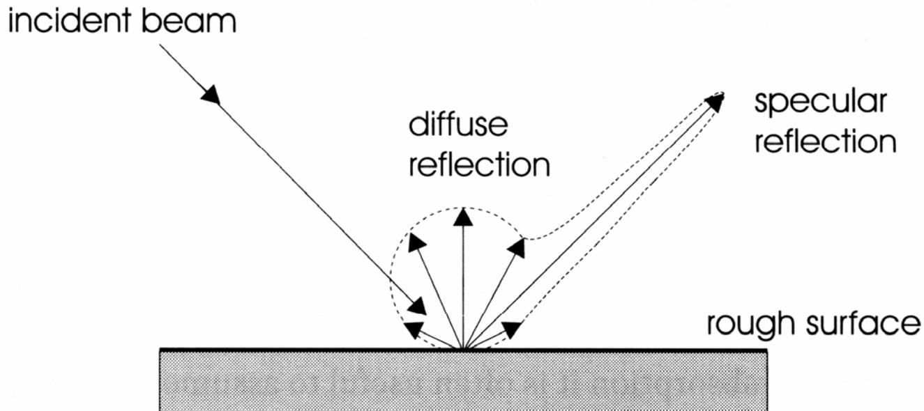
Reflection of light from a rough surface consists of two components, diffuse reflection and specular reflection. As the surface roughness increases the amount of diffuse reflection relative to the specular reflection increases. The ratio is an indication of surface gloss
