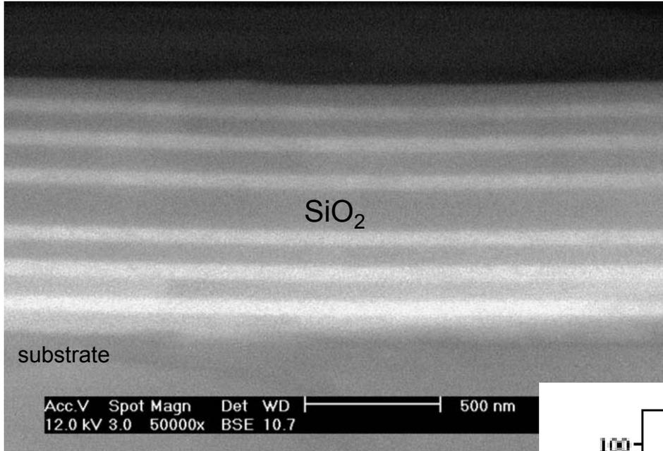
FEG-SEM cross-section micrograph (backscattered electron mode) of a single Fabry-Perot microcavity with a silica defect layer (dark color).
