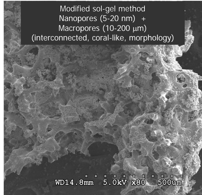
Scanning electron micrographs of glass samples of composition 70%  $\text{SiO}_2$  – 30%  $\text{CaO}$  (mol%), prepared by the normal (left) and modified (right) sol-gel technique
