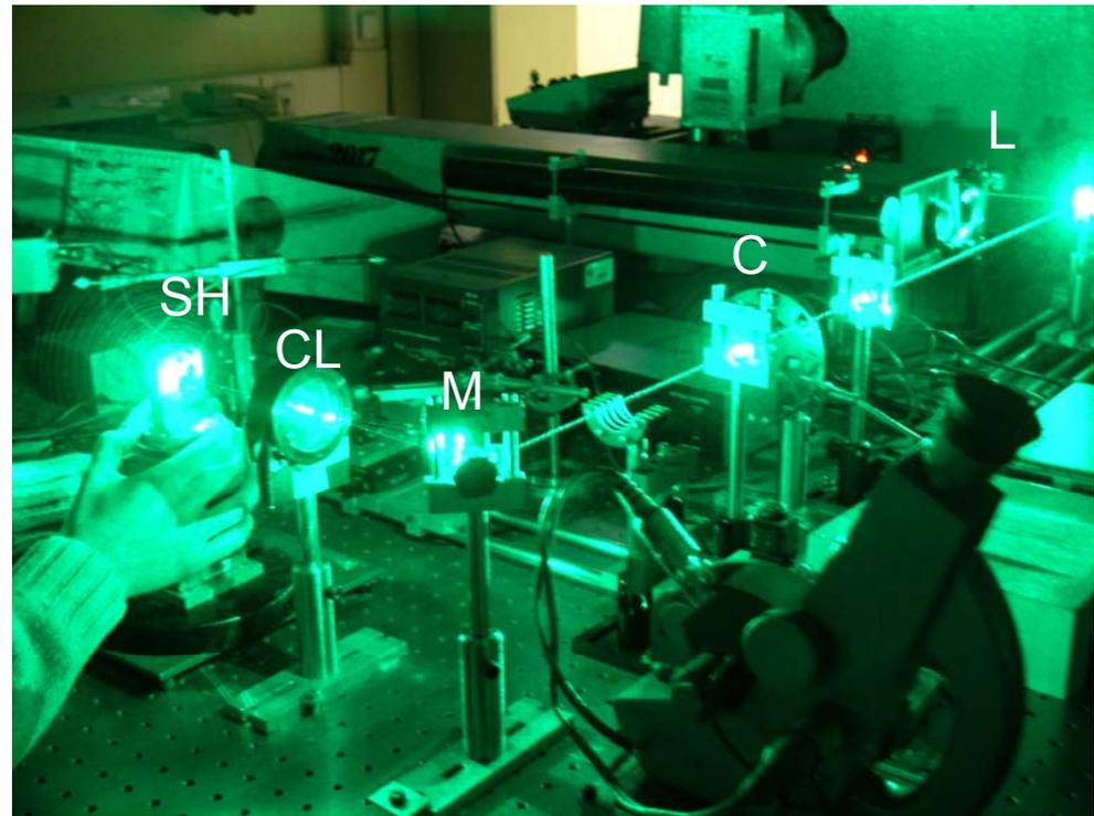
Laser beam used for photoluminescence measurements (M-mirror, CL-convergent lens, L-laser source, C-chopper, SH-sample holder)
