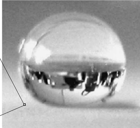
Thin films prepared with 0.075 g PAA. The contact angle for water was 151°.
