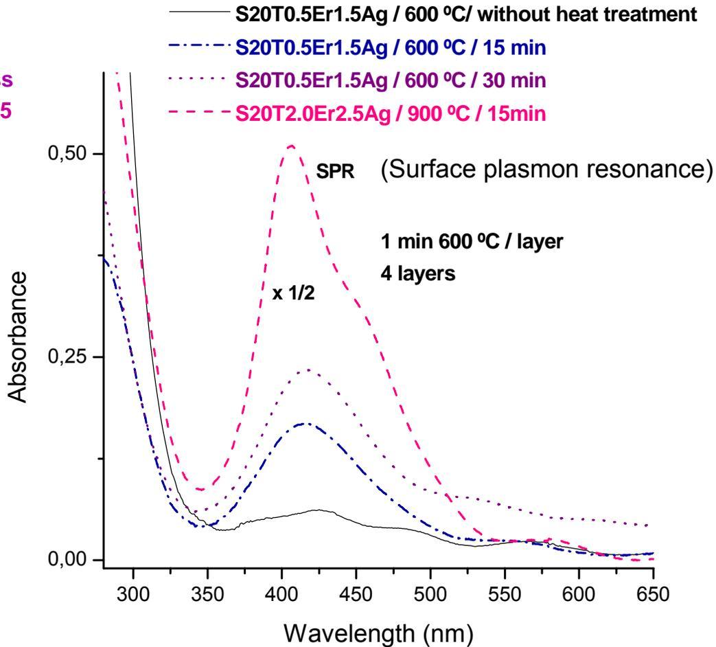
Er<sup>3+</sup> and Ag<sup>0</sup>-doped silica glass (pore doping with 0.15 M Er(NO<sub>3</sub>)<sub>3</sub> + 0.25 M AgNO<sub>3</sub> solution)
