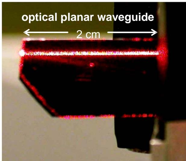
Light propagation in a planar waveguide of composition  $\text{SiO}_2\text{-TiO}_2\text{-Al}_2\text{O}_3$  (silica-on-silicon substrate; prism coupling).
