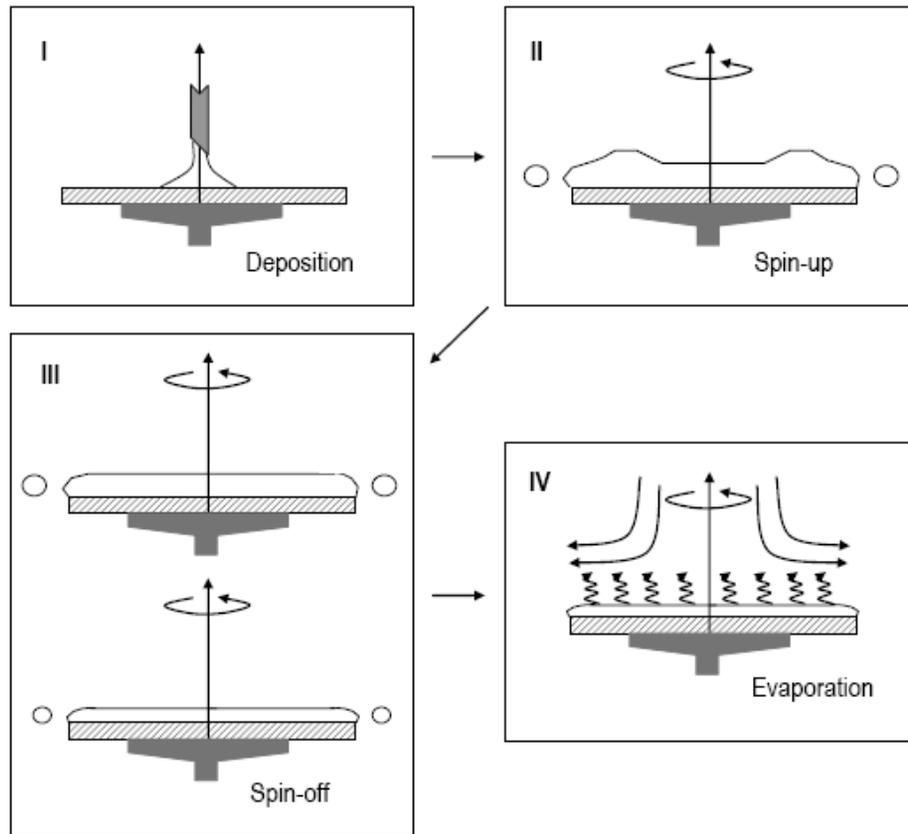
Stages of the spin-coating process: (I) deposition, (II) spin-up, (III) spin-off and (IV) evaporation. (not to scale).
