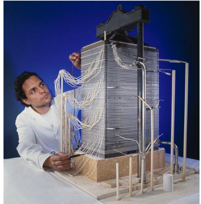
Fig. 6 SOFCs. Experimental unit. Julich Research Centre 13.3 kW
