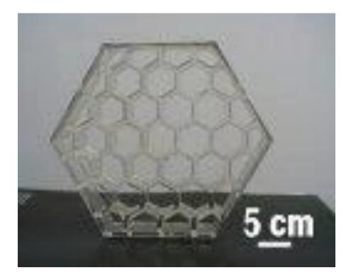
Equivalent of fused silica from sintered "Shoup Gels"
